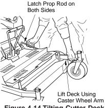
Figure 4-14 Tilting Cutter Deck
